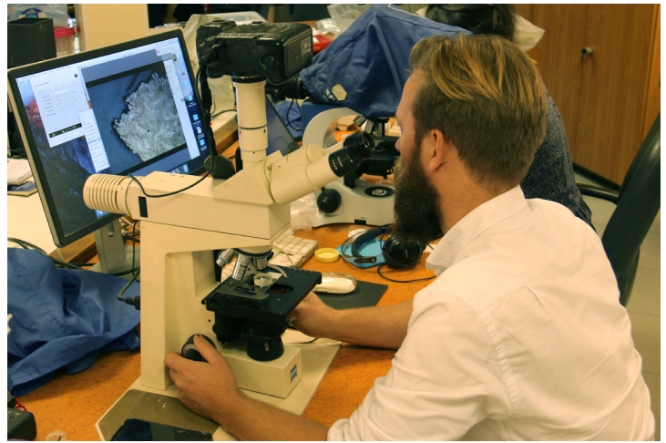
Jiří Kmošek documents the samples under a metallographic microscope. Photo by Martin Odler.
