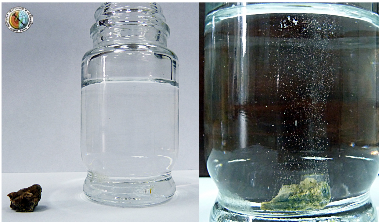
Photo of an experiment on the decomposition of limestone, taken from the blocks of the walls of the Saqsaywaman fortress, interacting with 70% acetic acid.
