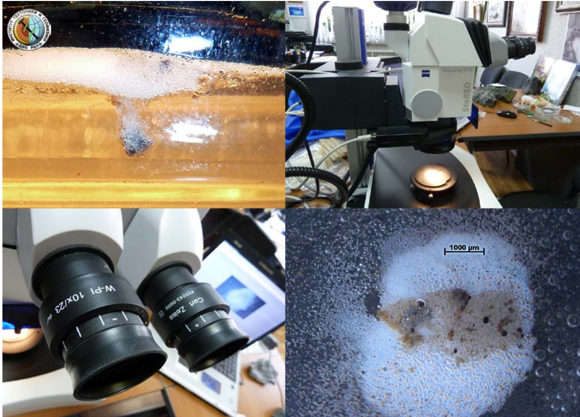
Photo of an experiment on the decomposition of limestone, taken from the blocks of the walls of the Saqsaywaman fortress, interacting with sulfuric acid.
