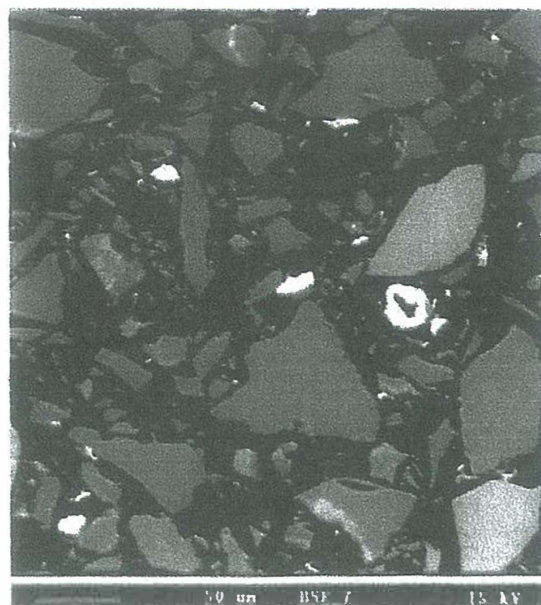
FIGURE 1. SEM photo of the core, made from hard limestone derived powder. Scale bar = 50 µm. (Photo courtesy of M.S. Tite and the Research Laboratory for Archaeology and the History of Art, Oxford University).
