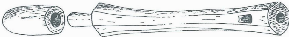
TOOLS. Figure 1. Kahun bow-driven drill stock, with its wooden drill cap. A tool can be removed by pushing a short stick into the ejection hole. (Drawn from Manchester Museum Catalogue number 23. Courtesy Denvs A. Stocks)
