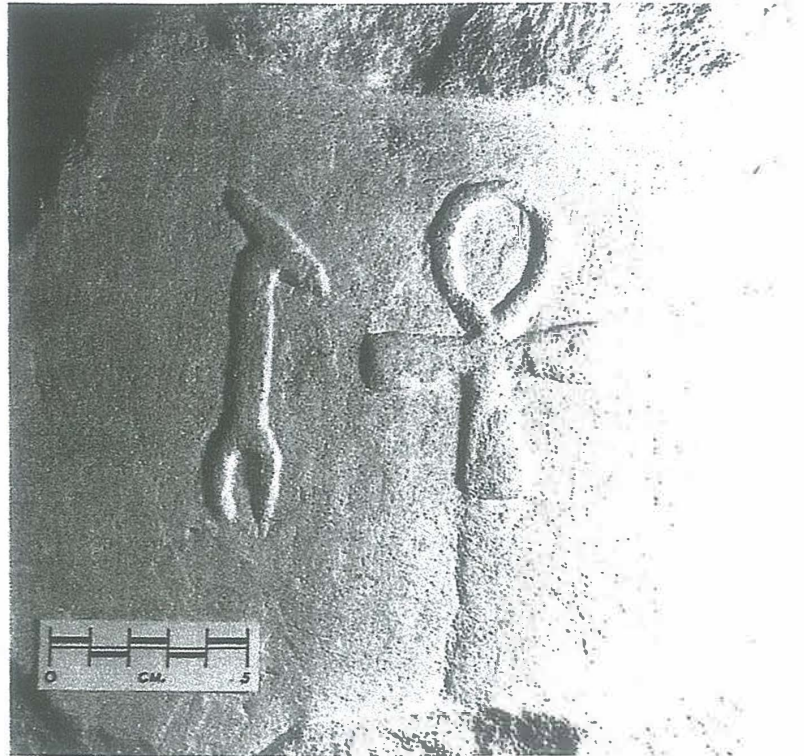
STONWORKING. Figure 2. Test bas relief in soft limestone, made by mallet-driven copper chisels. The edges were scraped by flint tools. (Courtesy Denys A. Stocks)
