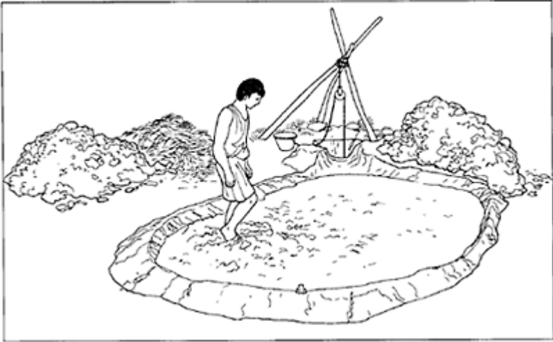
136 Mixing clay with straw as a defattening agent tempering by treading, in the preparation of puddled clay or unbaked bricks.
