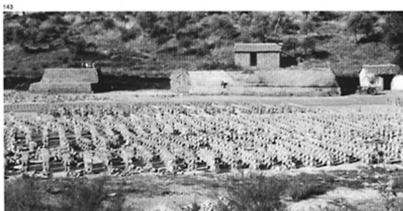
143 Brick-drying area and baking in a stack (behind) in the region of Mugla (Turkey).
