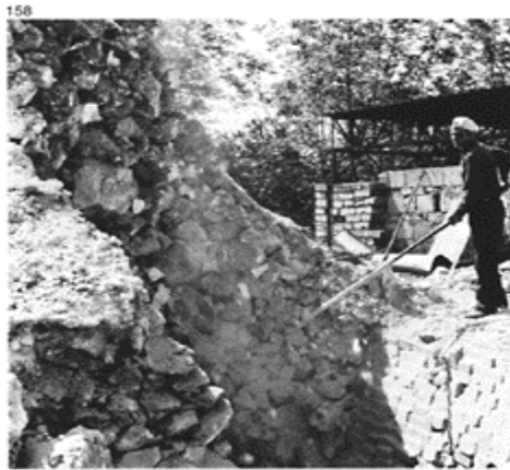
158 Opening of the kiln at Foca. The mass of quicklime is tackled with a mining iron by the lime burner Giovanni Molisse.
