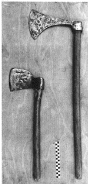
210 Two squaring axes (early twentieth century, France). ( Right ) Total length: 97cm; length of blade: 31.5cm. ( Left ) Total 20cm. length: 64cm; length of blade:
