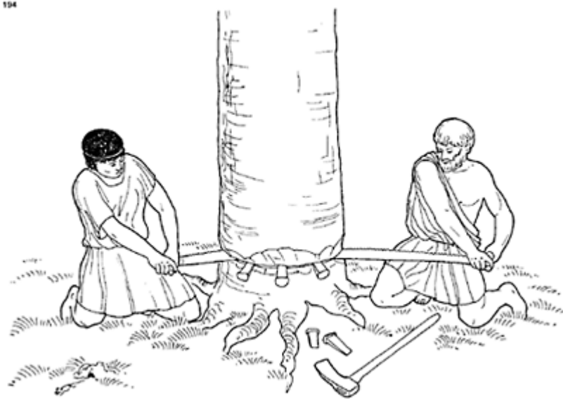
194 Cutting down a tree with a felling axe, two-handed cross-cut saw and wedges.
