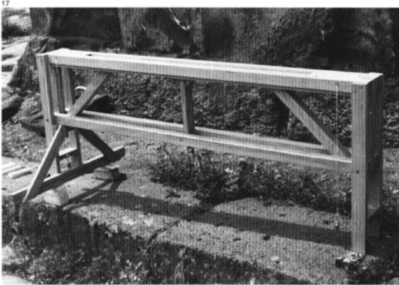
17 The reconstructed chorobates wedged into a horizontal position.
