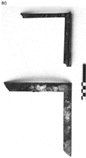
80 Two bronze squares found in Pompeii. The top one is a shouldering square. (National Museum, Naples.)
