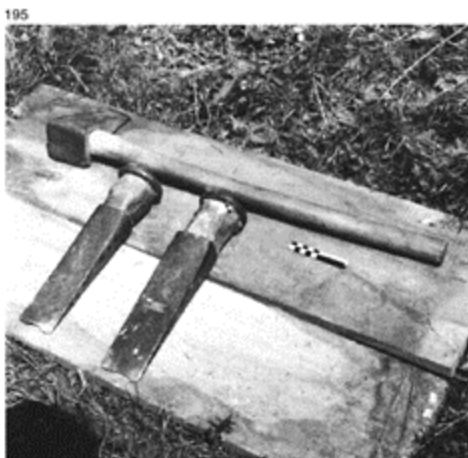
195 Splitting axe or cleaver and wedges, Vosges Mountains, twentieth century.
