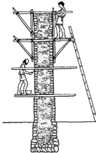
183 Socketed Scaffolding with transverse putlogs.
