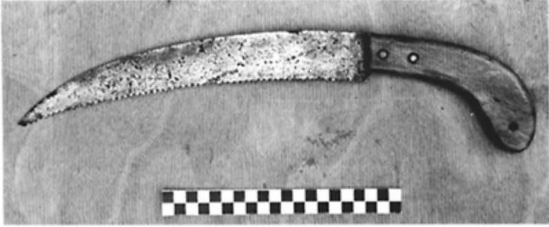
202 Small handsaw for limbing or cutting up small pieces of wood (early twentieth century). Compare with the two blades at the bottom of fig. 201.
