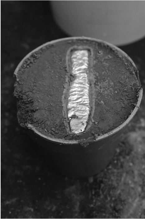
Figure 2.16 A cast copper adze blade
