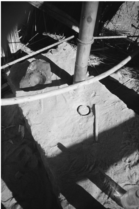
Figure 6.6 The copper tube used to drill out Khufu's granite sarcophagus was a little larger in diameter than this reconstructed tubular drill. The lubricated capstone is on the left
