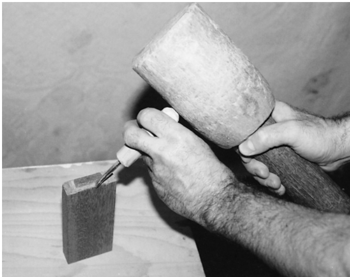
Figure 2.7 A mallet driving a replica woodworking chisel
