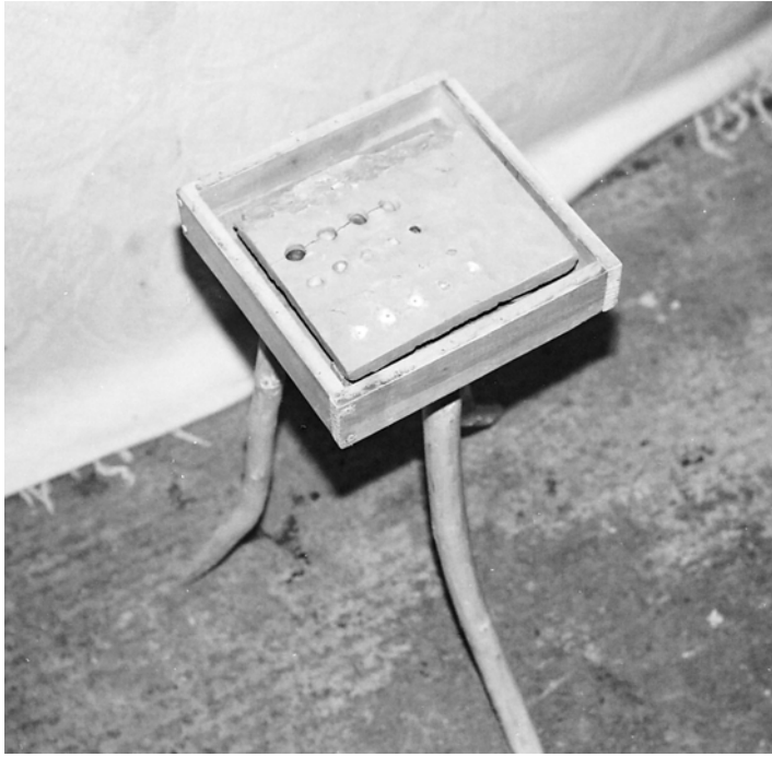
Figure 8.17 One of the test mud blocks, with trial stone pieces held firmly within it
