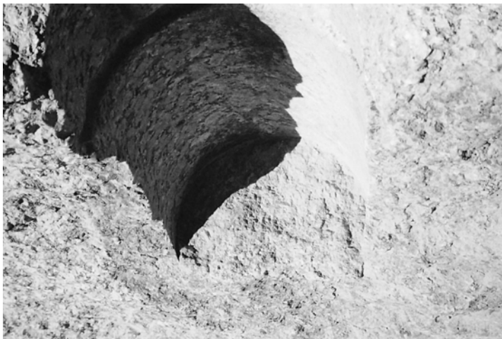
Figure 4.1 A large drill-hole in a rose granite block at Karnak, created by first drilling with a tube possessing a wall thickness of approximately 3 mm and then breaking out the core
