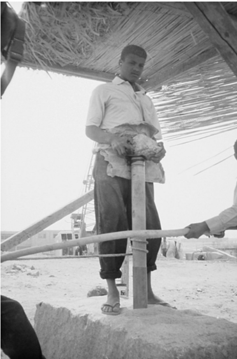
Figure 4.22 The bow-rope double turned around the drill-shaft
