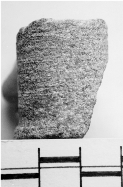
Figure 4.17 Striations cut into a stone core
