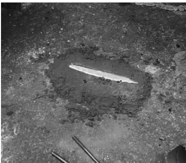
Figure 2.17 A cast copper woodcutting saw blade
