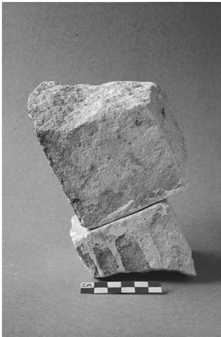
Figure 7.18 The lubricated sliding test using the prepared limestone blocks
