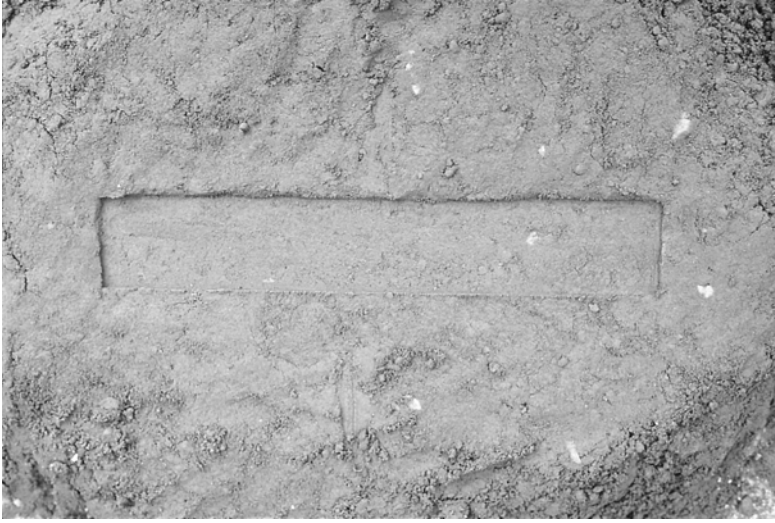
Figure 2.14 A mould pressed into damp sand for casting a flat-edged saw
