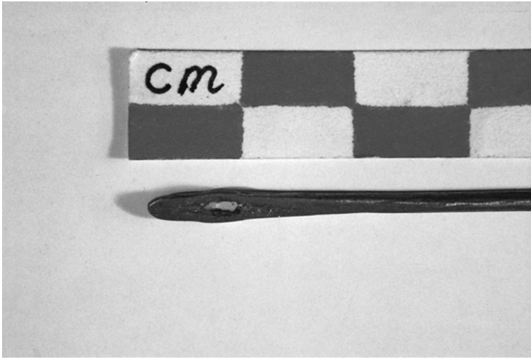
Figure 2.37 A hole punched through the head of an annealed copper needle
