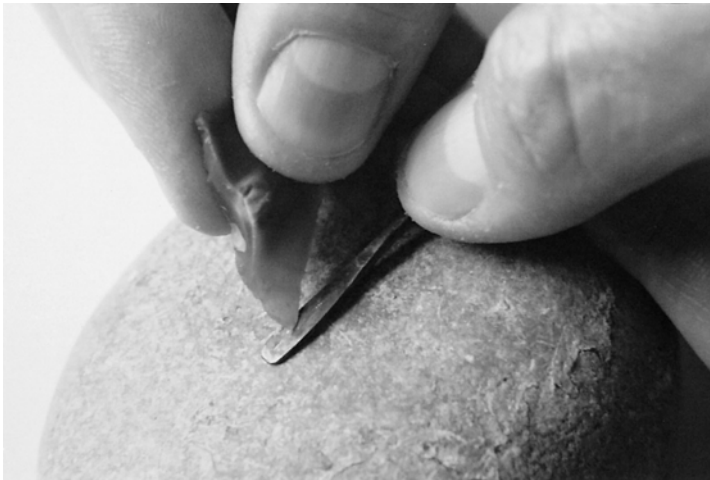
Figure 2.36 Scraping a depression into an annealed copper needle with a flint tool
