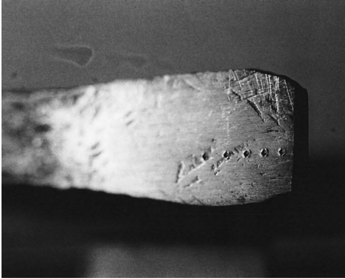
Figure 2.53 Hardness testing marks on a copper chisel's taper
