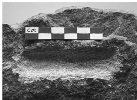
Figure 2.18 An experimental stone mould for casting a chisel
