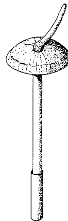
Figure 5.7 A proposed drilling version of the tool for making stone vessels, which has a copper tube force-fitted to its central shaft
