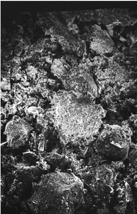
Figure 4.16 Scanning electron micrograph of finely ground granite derived powder. Many of the quartz and stone fragments are between 50 and 80 microns in size
