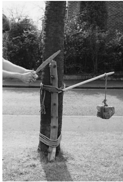
Figure 2.59 Using a saw with both hands while the wood remains firmly lashed to a post buried in the ground
