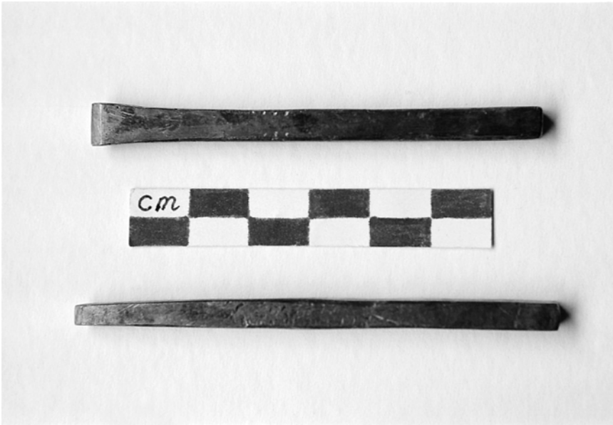
Figure 2.3 The shapes of the flat chisel (top) and the crosscut chisel (bottom) tapers
