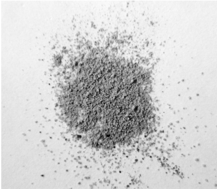
Figure 4.14 The waste product sand/copper/stone powder, obtained from drilling granite with a copper tube and sand
