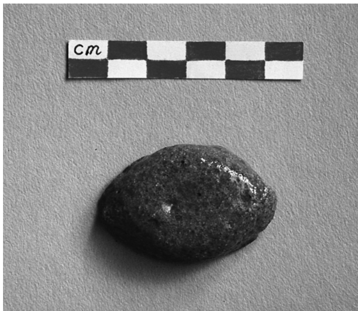
Figure 9.4 A glaze sample, made from the granite-derived powder
