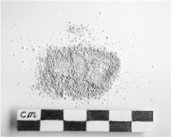
Figure 9.1 The whitish, waste product powder obtained from drilling hard limestone with a copper tube and sand
