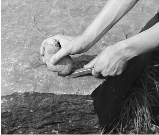
Figure 2.50 Hammering a bronze casting into a chisel
