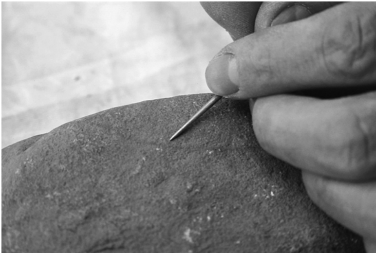
Figure 2.38 Sharpening the point of a hammer-hardened needle on a smooth piece of sandstone
