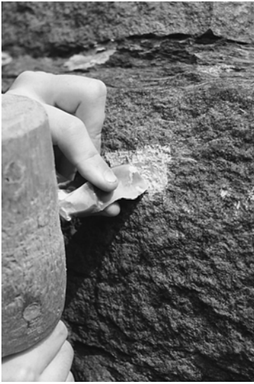
Figure 3.8 Chipping out pieces of hard sandstone with a mallet-driven flint chisel
